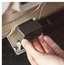
The AM-T22 plugs into the OBD socket in your vehicle.
