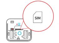
When the nano SIM card is inserted and the AM-T01 is ON, the LED will light up.
